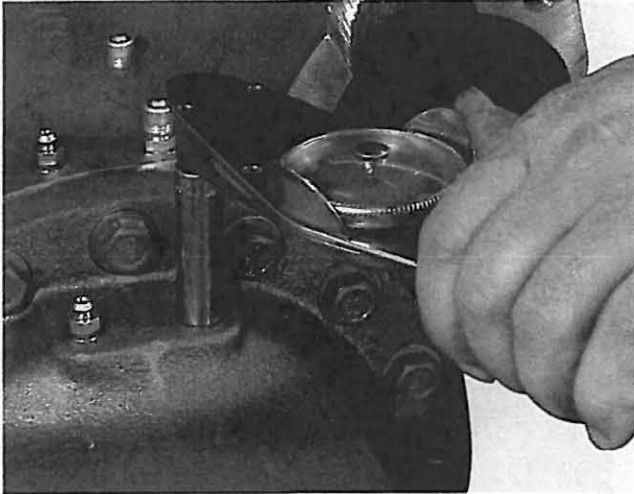
16. Torque fittings to 84-120 In. Lbs. (9.5-13.5 Nm).
